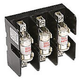
AutomationDirect fuse kit, 7-1/2hp and 10hp, 460/575 VAC, 3-phase, input side only, 200kA SCCR. For use with GS2/GS3-47P5, GS2-57P5, GS2-5010 AC drives.
