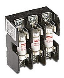
AutomationDirect fuse kit, 3hp and 5hp, 460/575 VAC, 3-phase, input side only, 200kA SCCR. For use with GS2/GS3-43P0, GS2-55P0 AC drives.
