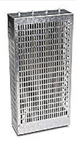
AutomationDirect braking resistor, 9600W, 13.6 ohm, NEMA 1, built-in temperature switch. For use with GS3-4100 AC drive. Requires GS-4DBU external braking unit.
