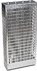
AutomationDirect braking resistor, 6 kW, 20 ohm, NEMA 1, built-in temperature switch. For use with multiple AC drives. Requires GS-4DBU external braking unit.
