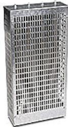
AutomationDirect braking resistor, 9.6 kW, 13.6 ohm, NEMA 1, built-in temperature switch. For use with multiple AC drives. Requires GS-4DBU external braking unit.
