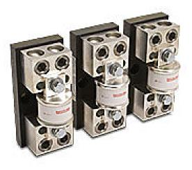
AutomationDirect fuse kit, 40hp, 460 VAC, 3-phase, input side only, 200kA SCCR. For use with GS3-4040 AC drive.
