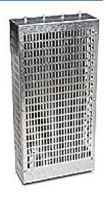
AutomationDirect braking resistor, 6000W, 20 ohm, NEMA 1, built-in temperature switch. For use with GS3-4040 AC drive. Requires GS-4DBU external braking unit.
