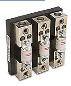
AutomationDirect fuse kit, 25hp, 460 VAC, 3-phase, input side only, 200kA SCCR. For use with GS3-4025 AC drive.
