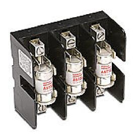
AutomationDirect fuse kit, 5hp, 230 VAC, 3-phase, input side only, 200kA SCCR. For use with GS2/GS3-25P0 AC drives.
