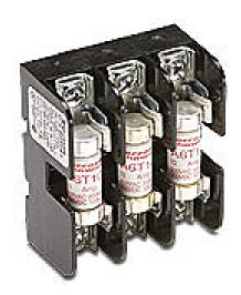
AutomationDirect fuse kit, 2hp, 230 VAC, 3-phase, input side only, 200kA SCCR. For use with GS1/GS2/GS3-22P0 AC drives.
