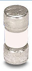
AutomationDirect spare fuse, 20A, 300 VAC, 200kA SCCR. Package of 5. For use with GS-20P5-FKIT-1P AC drive fuse kit.
