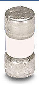
AutomationDirect spare fuse, 15A, 300 VAC, 200kA SCCR. Package of 5. For use with GS-20P2-FKIT-1P AC drive fuse kit.
