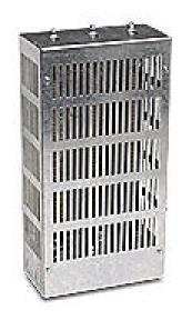
AutomationDirect braking resistor, 3000W, 10 ohm, NEMA 1, built-in temperature switch. For use with GS3-2020 AC drive. Requires GS-2DBU external braking unit.
