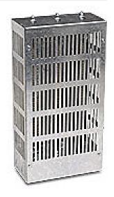
AutomationDirect braking resistor, 2400W, 13.6 ohm, NEMA 1, built-in temperature switch. For use with GS3-2015 AC drive.
