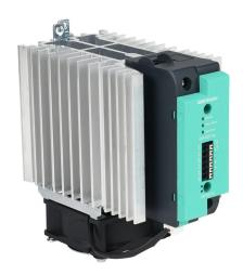
Gefran solid state relay with fan, 35mm DIN rail mount, 6-32 VDC input voltage, SPST, (1) N.O. SCR, 90A contact rating, 24-600 VAC load voltage, push-in spring, overvoltage and thermal protection. Thermal/load interruption alarm.
