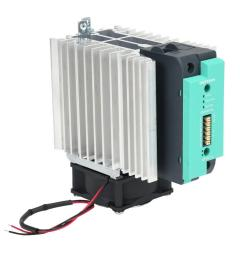
Gefran solid state relay with fan, 35mm DIN rail mount, 6-32 VDC input voltage, SPST, (1) N.O. SCR, 90A contact rating, 24-600 VAC load voltage, push-in spring, overvoltage and thermal protection, external 24 VDC required. Thermal/load interruption alarm.
