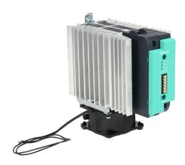
Gefran solid state relay with fan, 35mm DIN rail mount, 6-32 VDC input voltage, SPST, (1) N.O. SCR, 90A contact rating, 24-600 VAC load voltage, push-in spring, overvoltage and thermal protection, external 115 VAC required. Thermal/load interruption alarm.
