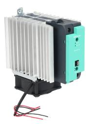
Gefran solid state relay with fan, 35mm DIN rail mount, 6-32 VDC input voltage, SPST, (1) N.O. SCR, 90A contact rating, 24-600 VAC load voltage, push-in spring, overvoltage and thermal protection, external 24 VDC required.
