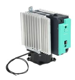
Gefran solid state relay with fan, 35mm DIN rail mount, 6-32 VDC input voltage, SPST, (1) N.O. SCR, 90A contact rating, 24-600 VAC load voltage, push-in spring, overvoltage and thermal protection, external 115 VAC required.
