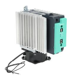
Gefran solid state relay with fan, 35mm DIN rail mount, 20-260 VAC input voltage, SPST, (1) N.O. SCR, 90A contact rating, 24-600 VAC load voltage, push-in spring, overvoltage and thermal protection, external 115 VAC required. Thermal alarm.
