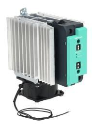
Gefran solid state relay with fan, 35mm DIN rail mount, 20-260 VAC input voltage, SPST, (1) N.O. SCR, 90A contact rating, 24-600 VAC load voltage, push-in spring, overvoltage and thermal protection, external 230 VAC required. Thermal alarm.
