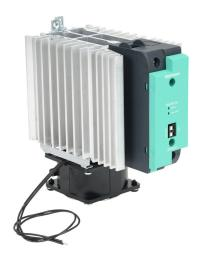
Gefran solid state relay with fan, 35mm DIN rail mount, 20-260 VAC input voltage, SPST, (1) N.O. SCR, 90A contact rating, 24-600 VAC load voltage, push-in spring, overvoltage and thermal protection, external 115 VAC required.
