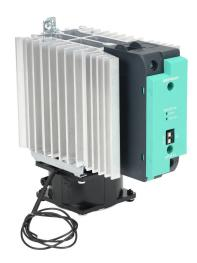
Gefran solid state relay with fan, 35mm DIN rail mount, 20-260 VAC input voltage, SPST, (1) N.O. SCR, 90A contact rating, 24-600 VAC load voltage, push-in spring, overvoltage and thermal protection, external 230 VAC required.
