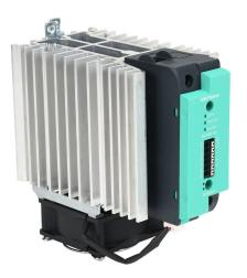
Gefran solid state relay with fan, 35mm DIN rail mount, 6-32 VDC input voltage, SPST, (1) N.O. SCR, 90A contact rating, 24-480 VAC load voltage, push-in spring, overvoltage and thermal protection. Thermal/load interruption alarm.
