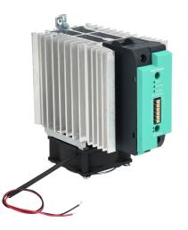
Gefran solid state relay with fan, 35mm DIN rail mount, 6-32 VDC input voltage, SPST, (1) N.O. SCR, 90A contact rating, 24-480 VAC load voltage, push-in spring, overvoltage and thermal protection, external 24 VDC required. Thermal/load interruption alarm.
