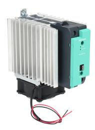
Gefran solid state relay with fan, 35mm DIN rail mount, 6-32 VDC input voltage, SPST, (1) N.O. SCR, 90A contact rating, 24-480 VAC load voltage, push-in spring, overvoltage and thermal protection, external 24 VDC required.
