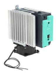
Gefran solid state relay with fan, 35mm DIN rail mount, 6-32 VDC input voltage, SPST, (1) N.O. SCR, 90A contact rating, 24-480 VAC load voltage, push-in spring, overvoltage and thermal protection, external 230 VAC required.
