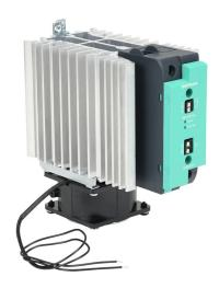
Gefran solid state relay with fan, 35mm DIN rail mount, 20-260 VAC input voltage, SPST, (1) N.O. SCR, 90A contact rating, 24-480 VAC load voltage, push-in spring, overvoltage and thermal protection, external 115 VAC required. Thermal alarm.
