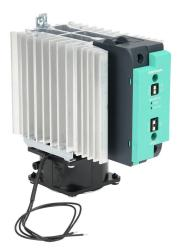
Gefran solid state relay with fan, 35mm DIN rail mount, 20-260 VAC input voltage, SPST, (1) N.O. SCR, 90A contact rating, 24-480 VAC load voltage, push-in spring, overvoltage and thermal protection, external 230 VAC required. Thermal alarm.
