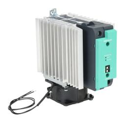
Gefran solid state relay with fan, 35mm DIN rail mount, 20-260 VAC input voltage, SPST, (1) N.O. SCR, 90A contact rating, 24-480 VAC load voltage, push-in spring, overvoltage and thermal protection, external 115 VAC required.
