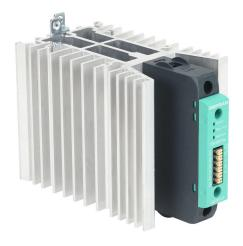
Gefran solid state relay, 35mm DIN rail mount, 6-32 VDC input voltage, SPST, (1) N.O. SCR, 75A contact rating, 24-600 VAC load voltage, push-in spring, overvoltage and thermal protection. Thermal/load interruption alarm.
