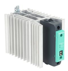
Gefran solid state relay, 35mm DIN rail mount, 20-260 VAC input voltage, SPST, (1) N.O. SCR, 75A contact rating, 24-600 VAC load voltage, push-in spring, overvoltage and thermal protection.
