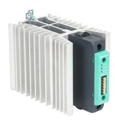
Gefran solid state relay, 35mm DIN rail mount, 6-32 VDC input voltage, SPST, (1) N.O. SCR, 75A contact rating, 24-480 VAC load voltage, push-in spring, overvoltage and thermal protection. Thermal/load interruption alarm.
