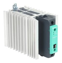
Gefran solid state relay, 35mm DIN rail mount, 6-32 VDC input voltage, SPST, (1) N.O. SCR, 75A contact rating, 24-480 VAC load voltage, push-in spring, overvoltage and thermal protection.
