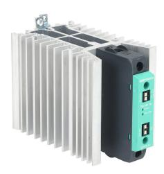
Gefran solid state relay, 35mm DIN rail mount, 20-260 VAC input voltage, SPST, (1) N.O. SCR, 75A contact rating, 24-480 VAC load voltage, push-in spring, overvoltage and thermal protection. Thermal alarm.
