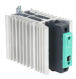
Gefran solid state relay, 35mm DIN rail mount, 6-32 VDC input voltage, SPST, (1) N.O. SCR, 60A contact rating, 24-600 VAC load voltage, push-in spring, overvoltage and thermal protection.
