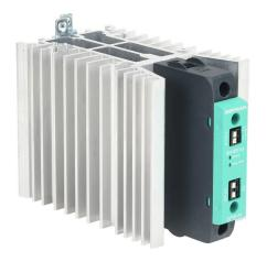
Gefran solid state relay, 35mm DIN rail mount, 20-260 VAC input voltage, SPST, (1) N.O. SCR, 60A contact rating, 24-600 VAC load voltage, push-in spring, overvoltage and thermal protection. Thermal alarm.
