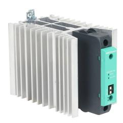
Gefran solid state relay, 35mm DIN rail mount, 20-260 VAC input voltage, SPST, (1) N.O. SCR, 60A contact rating, 24-600 VAC load voltage, push-in spring, overvoltage and thermal protection.
