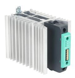
Gefran solid state relay, 35mm DIN rail mount, 6-32 VDC input voltage, SPST, (1) N.O. SCR, 60A contact rating, 24-480 VAC load voltage, push-in spring, overvoltage and thermal protection. Thermal/load interruption alarm.
