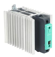
Gefran solid state relay, 35mm DIN rail mount, 6-32 VDC input voltage, SPST, (1) N.O. SCR, 60A contact rating, 24-480 VAC load voltage, push-in spring, overvoltage and thermal protection.
