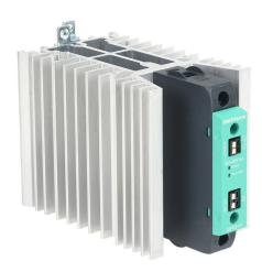
Gefran solid state relay, 35mm DIN rail mount, 20-260 VAC input voltage, SPST, (1) N.O. SCR, 60A contact rating, 24-480 VAC load voltage, push-in spring, overvoltage and thermal protection. Thermal alarm.
