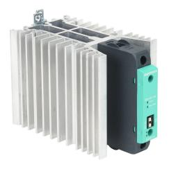
Gefran solid state relay, 35mm DIN rail mount, 20-260 VAC input voltage, SPST, (1) N.O. SCR, 60A contact rating, 24-480 VAC load voltage, push-in spring, overvoltage and thermal protection.
