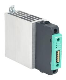
Gefran solid state relay, 35mm DIN rail mount, 6-32 VDC input voltage, SPST, (1) N.O. SCR, 50A contact rating, 24-600 VAC load voltage, push-in spring, overvoltage and thermal protection. Thermal/load interruption alarm.
