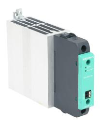
Gefran solid state relay, 35mm DIN rail mount, 6-32 VDC input voltage, SPST, (1) N.O. SCR, 50A contact rating, 24-600 VAC load voltage, push-in spring, overvoltage and thermal protection.
