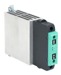
Gefran solid state relay, 35mm DIN rail mount, 20-260 VAC input voltage, SPST, (1) N.O. SCR, 50A contact rating, 24-600 VAC load voltage, push-in spring, overvoltage and thermal protection. Thermal alarm.
