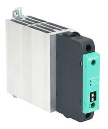
Gefran solid state relay, 35mm DIN rail mount, 20-260 VAC input voltage, SPST, (1) N.O. SCR, 50A contact rating, 24-600 VAC load voltage, push-in spring, overvoltage and thermal protection.
