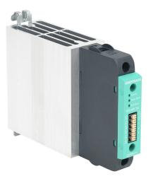
Gefran solid state relay, 35mm DIN rail mount, 6-32 VDC input voltage, SPST, (1) N.O. SCR, 50A contact rating, 24-480 VAC load voltage, push-in spring, overvoltage and thermal protection. Thermal/load interruption alarm.
