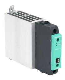
Gefran solid state relay, 35mm DIN rail mount, 6-32 VDC input voltage, SPST, (1) N.O. SCR, 50A contact rating, 24-480 VAC load voltage, push-in spring, overvoltage and thermal protection.
