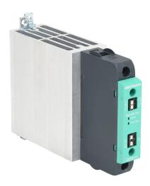
Gefran solid state relay, 35mm DIN rail mount, 20-260 VAC input voltage, SPST, (1) N.O. SCR, 50A contact rating, 24-480 VAC load voltage, push-in spring, overvoltage and thermal protection. Thermal alarm.
