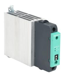
Gefran solid state relay, 35mm DIN rail mount, 20-260 VAC input voltage, SPST, (1) N.O. SCR, 50A contact rating, 24-480 VAC load voltage, push-in spring, overvoltage and thermal protection.
